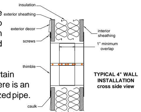
4. Slide the interior portion of the Thimble into the inside hole. Be certain the interior and exterior Thimble halves overlap at least 1 inch. If there is an insufficient overlap extend the interior portion with single wall galvanized pipe.
